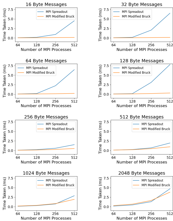
Figure 4: Weak scaling study comparing MPI all-to-all methods, our basis for investigating Bruck performance in NCCL. The Bruck implementation performs significantly better for small-sized messages and at larger scales than spread-out. This advantage, however, becomes much smaller for large-sized messages.
